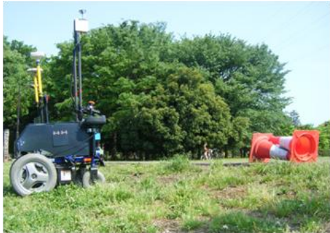
Fig.4 Obstacle detection by 2 LRFs
